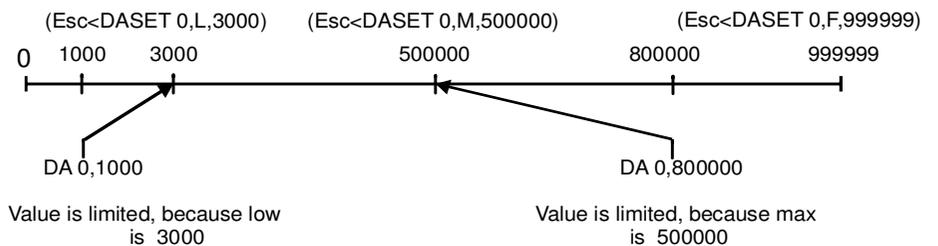
Ps. When autoscaling: Using a unipolar DAC, the initially Offset value must always be negative and the gain a bit too high. From version SCC108, a bipolar DAC can be attached, that is, the Offset may be initially either positive or negative but the gain must still be a bit too high. On bipolar DACs, the gain can only be auto adjusted at +100%.
